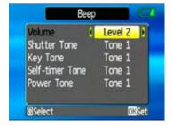
3. Use the **Left/Right** navigation buttons to adjust the volume and change each tone style. Then press the button to confirm.
